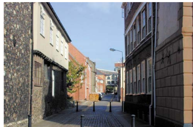
Use of bollards to prevent vehicles from passing but to promote pedestrian and cyclist permeability
