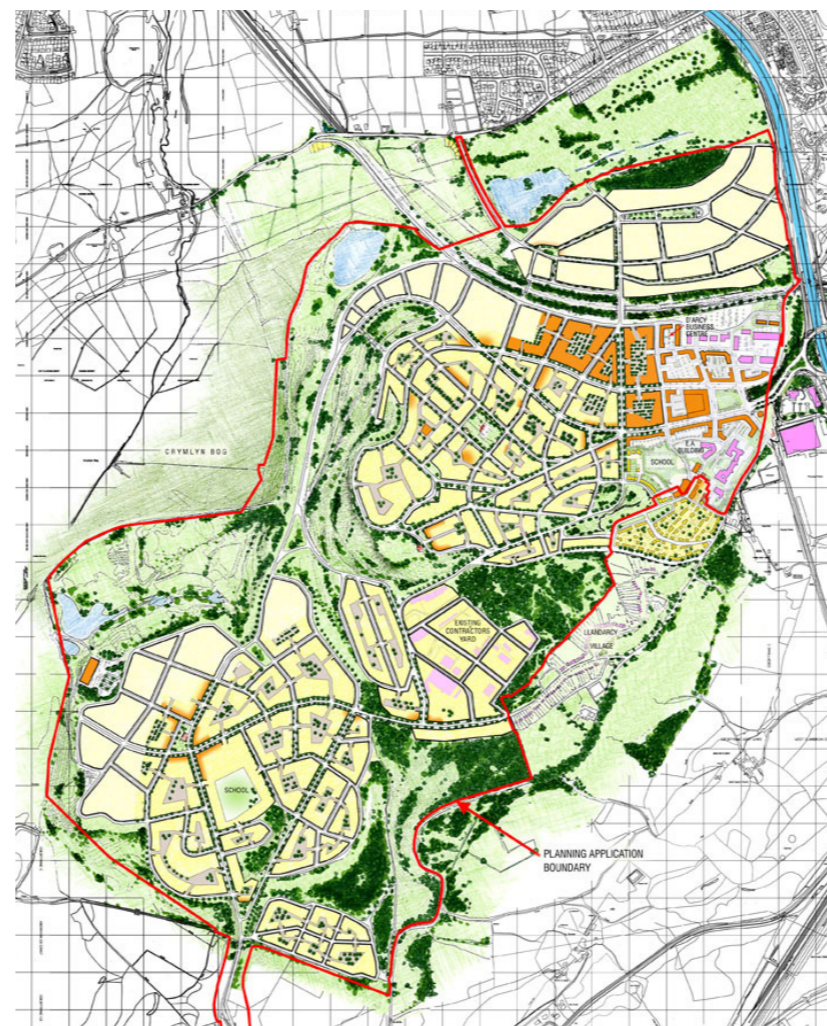
Figure 37: This plan indicates the block layout and typology. It also takes into account the natural features and topography of the site
