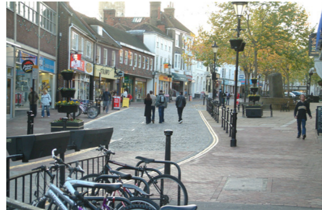
Local High Street which provides wide pavements, integrated traffic calming measures, changing textures and cycle parking facilities
