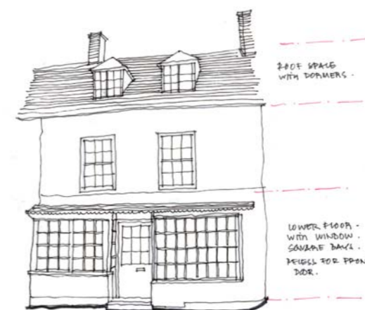
Figure 158: Typology of building elevations found on the Towcester High Street, highlighting their characteristic features
