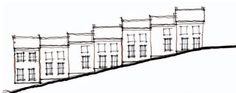
Figure 210: Indicative section through a street that steeply slopes resulting in a stepping pattern evident in the terraced houses
