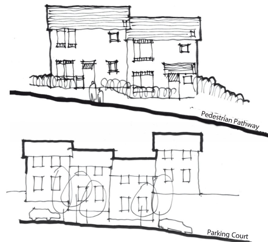
Figure 219: In these examples from the suburbs of Northampton, the natural topography of the land has been utilized to create a degree of separation between the private realm of the houses and the public realm of the street, parking courts and pedestrian walkways
