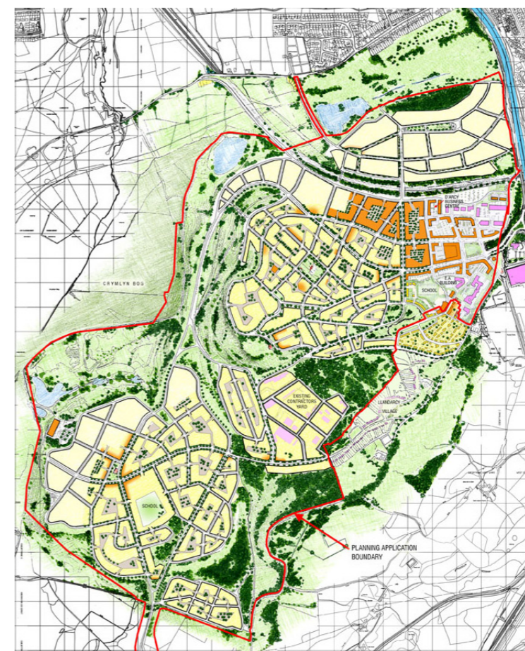
Figure 226 - Coed Darcy Masterplan - The blocks are laid out in an orthogonal manner where the streets either follow the contours or run across them, thereby terminating in wider views of the surrounding countryside
