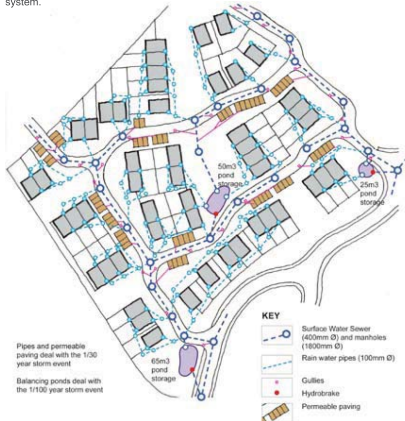
Figure 5.1.11 An “end of pipe” solution, whereby traditional gullies and pipes are partially replaced by an element of permeable paving, with the main attenuation capacity being provided by oversized pipes with detention ponds at the end of the system.
