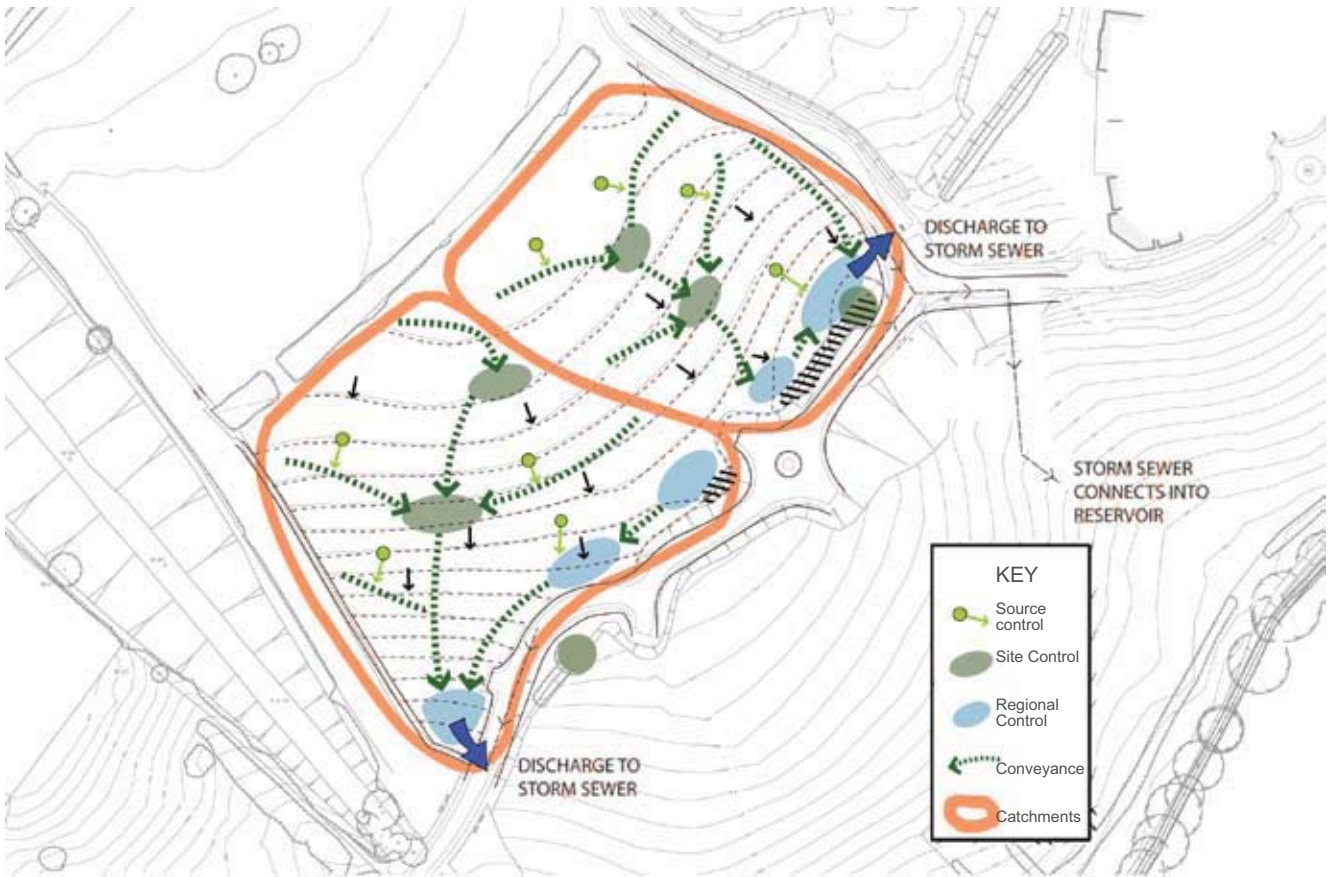
Figure 5.1.1: The site can be split into two sub-catchments, each with SUDS controls from the top of the site (source and site controls) to the bottom of the site (regional controls)
