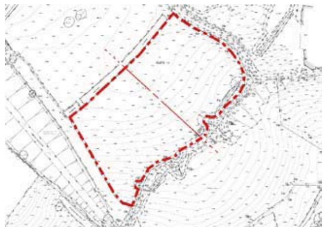
Figure 5.1.4 (above): Reviewing the topography shown in the plan will start to identify the natural slope of the existing land. The site can be notionally split into two to demonstrate two 50-unit neighbourhood modules
