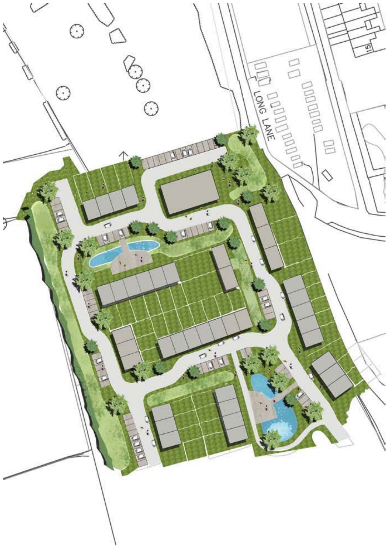
Figure 5.2.8: Phase 1 in detail - illustrating that it is possible to be flexible in the detailed design without damaging the overall infrastructure concept. In this case, the SUDS features changed position from the outline masterplan, whilst maintaining the necessary source and site features
