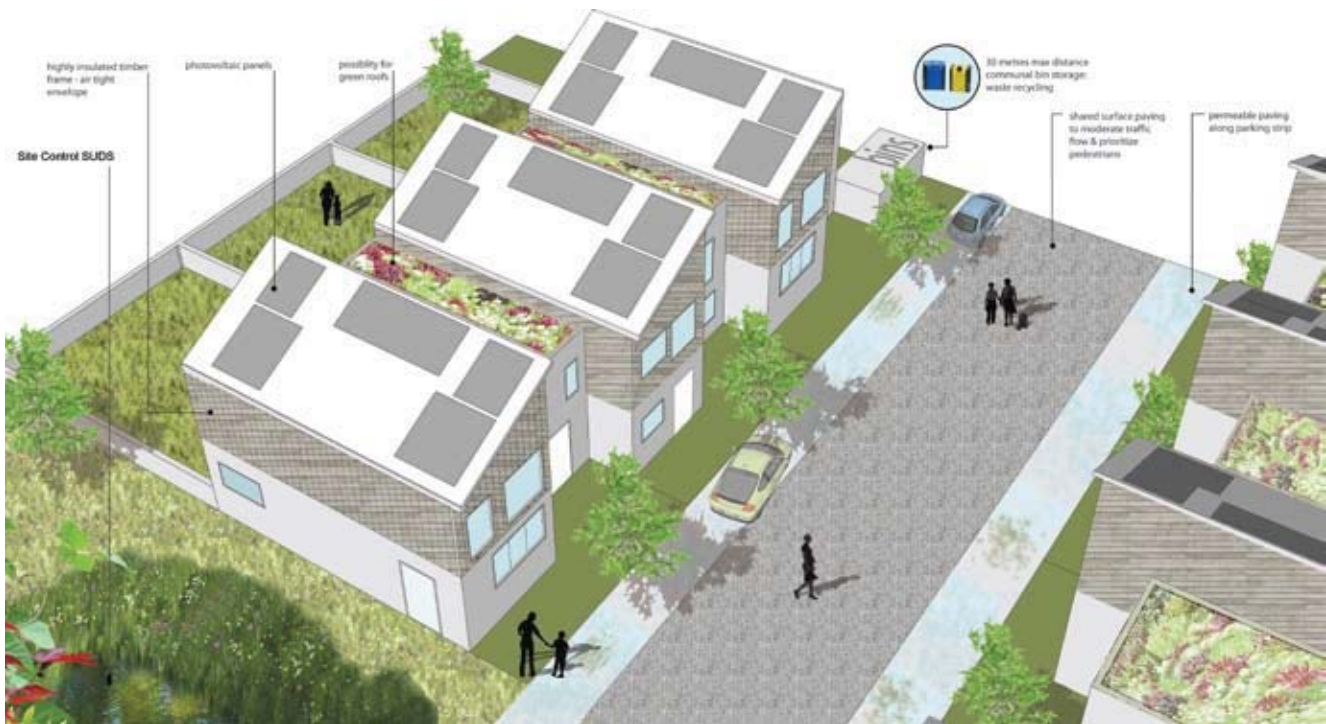
Figure 5.1.7: An image of the housing units, illustrating the integration of the three infrastructures. These units could equally be an apartment block at a higher density
