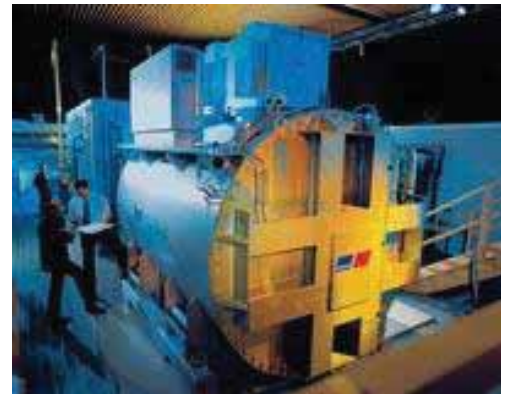
Figure 5.2: Fuel Cell CHP – MTU Hot Module (source: MTU CFC Solutions GmbH)
