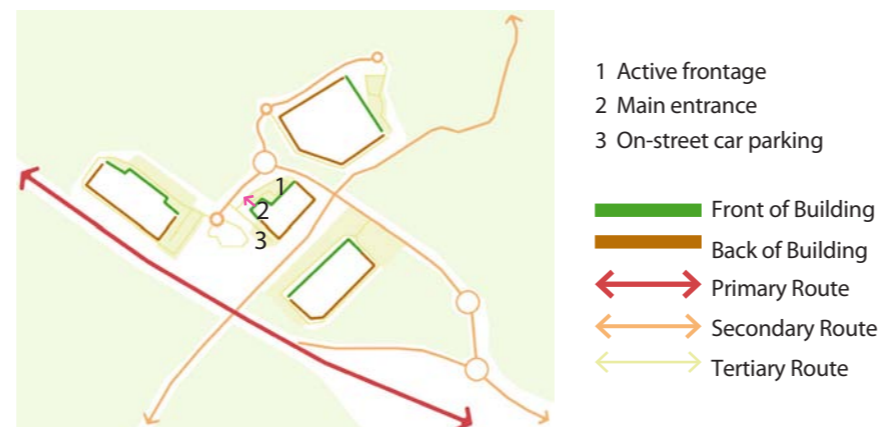
Figure 250: Concept image showing the relationship of the Levi Strauss Ltd Office Building to its surroundings and within the movement hierarchy
