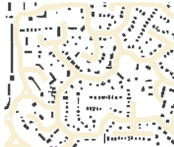
Figure 117: Figure ground of a suburban neighbourhood highlighting the loose nature of the layout with streets that terminate in cul de sacs
